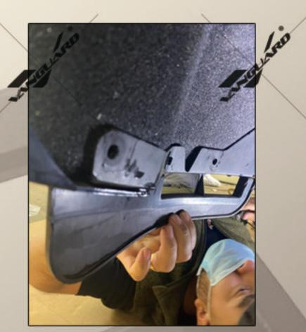
1.Remove the mudguard under the car first.
