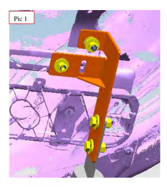
Step 3: Install the bull bar on the brackets and then adjust them to the proper positions. Step 4: Check if all hard ware are installed and then fasten all to complete the installation.
