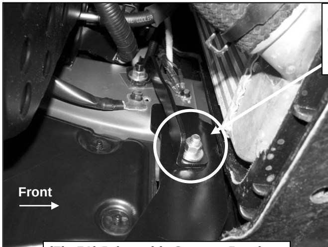
(Fig 5A) Driver side Support Bracket. NOTE: Only required for driver side
