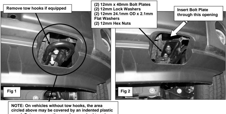
circled above may be covered by an indented plastic panel. Cut or remove the panel as required to gain access to the front of the frame rail to allow bottom brackets to pass through the bumper cover.
