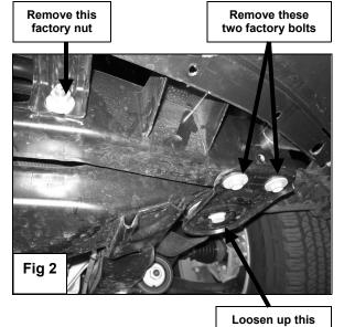
Slide Mounting Bracket between cross member bar and radiator support bracket
