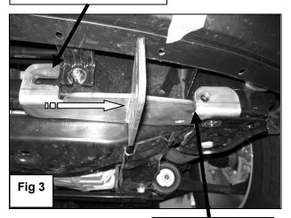
Slide Mounting Bracket between motor mount bushing
