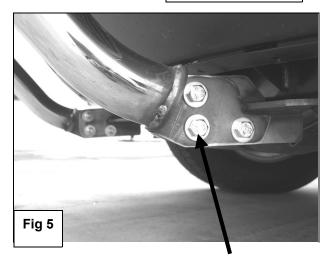
12mm x 30mm Hex Head Bolts 12mm Nylock Nuts 12mm Flat Washers
