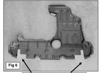
Cut out the sections illustrated to clear the Mounting Brackets (Pictured for example only, actual area to cut may be different) Hold the plastic splash guard up to the bottom of the brackets. Trace location of brackets onto the inside of the splash guard. Picture used for example only
