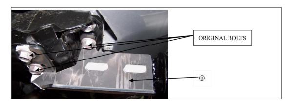
3、INSTALL O WITH BRACKETS AND TIGHTEN BOLTS. SEE THE PICTURE BELOW.
