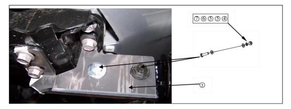
STEP THREE: MAKRE SURE BOLTS ARE TIGHTENED AND THE GRILL GUARD IS FIXING STRONG ENOUGH.
