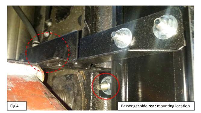
STEP5: Next, move on to the passenger side rear and insert two drop pins into the factory holes. Select passenger side rear mounting bracket and secure it with flat washers, lock washers and nuts. Do not tighten hardware at this time. (Fig4)
