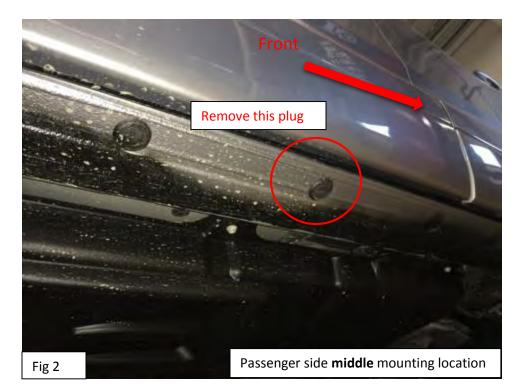
STEP3: Next, locate and remove the middle rubber plug. (Fig2)
