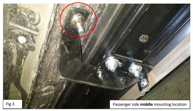
STEP4: Insert a drop pin into the factory hole. Select passenger side middle mounting bracket and secure it with a flat washer, a lock washer and a nut. Do not tighten hardware at this time. (Fig3)
