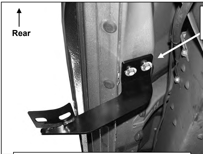
(Fig 5) Driver/Left Rear Bracket installed
