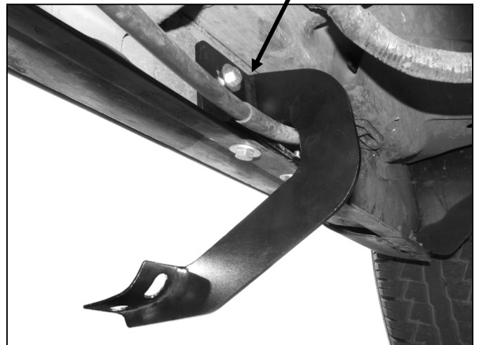
(Fig 2) Driver side-front Mounting Bracket location
