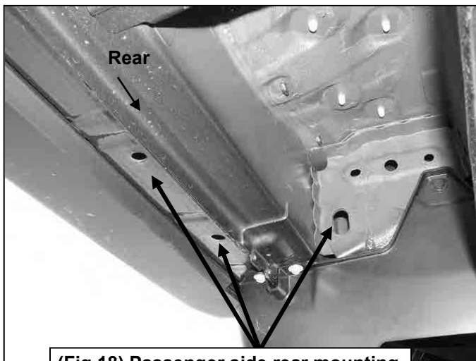
(Fig 18) Passenger side rear mounting location pictured from below. Remove rubber plugs from factory holes
