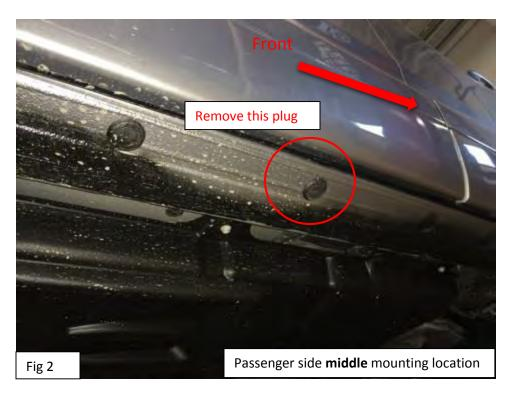
STEP3: Next, locate and remove the middle rubber plug. (Fig2)
