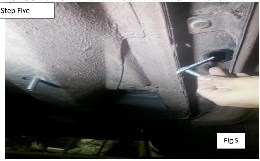
INSERT ANOTHER DROP IN FOR THE FRONT SUPPORT. AND USE ANOTHER DROP IN FOR THE REAR SUPPORT. USE THE FACTORY OPEN HOLE FOR THE REAR DROP IN.
