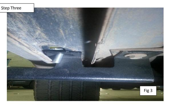
MOUNT UP REAR BRACKET USING THE DROP IN SCREW. REUSE THE FACTORY SCREW TO MOUNT THE REAR SIDE OF THE BRACKET.
