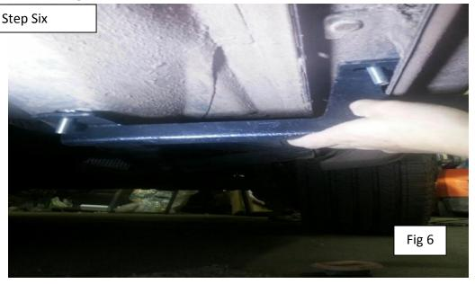
MOUNT FRONT BRACKET. USE FLAT WASHER, LOCK WASHER AND NUT FOR BOTH.USE EXTRA SPACERS IF NECESSARY IF YOU NEED TO MAKE
