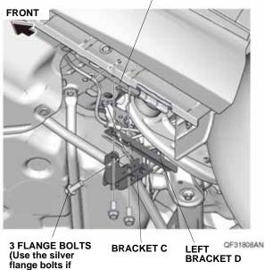
included in the kit.) (Loosely secure.) 26. With the help of an assistant, loosely secure the left running board to bracket A, bracket B, bracket C, and left bracket D with 13 flange bolts. NOTE: If there are black and silver flange bolts in the kit, use six black flange bolts and seven silver flange bolts as shown.
