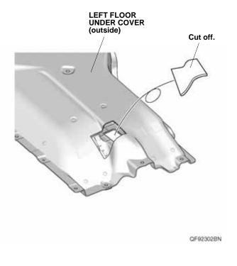
15. Using a utility knife, cut off the left floor under cover as shown.
