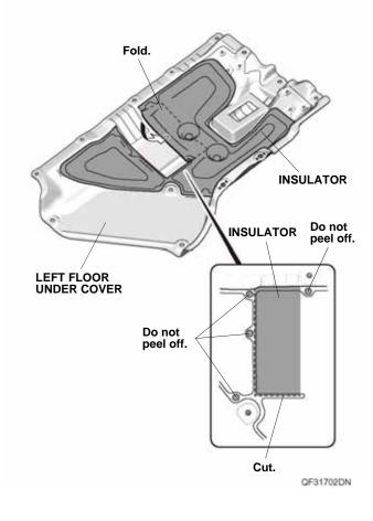
9. Using a utility knife, cut the insulator on the right floor under cover and fold it into the inside of the insulator as shown.
