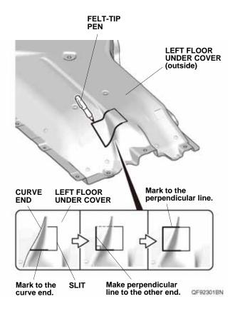
14. Using a utility knife, cut off the left floor under cover along the mark.
