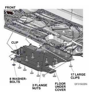
If the vehicle is equipped with the insulator on the floor under cover, continue with step 2; otherwise, go to step 4.
