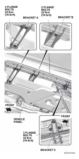
Secure the left running board to bracket A, bracket B, bracket C, and left bracket D with 13 flange bolts. Torque the flange bolts to 22 N·m (16 lb·ft).
