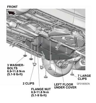
23. Install the right floor under cover. Torque the flange nut and washer-bolts to 6.9-11.8 N·m (5.1-9 lb·ft).
