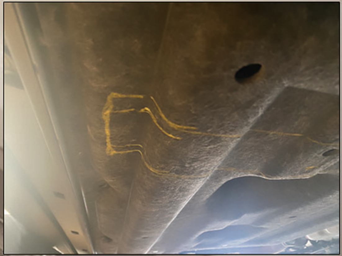
2. Draw the installation position of the bracket on the fender.
