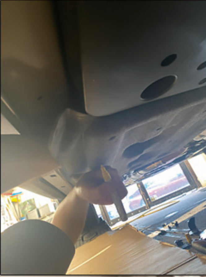
2. Draw the installation position of the bracket on the fender.
