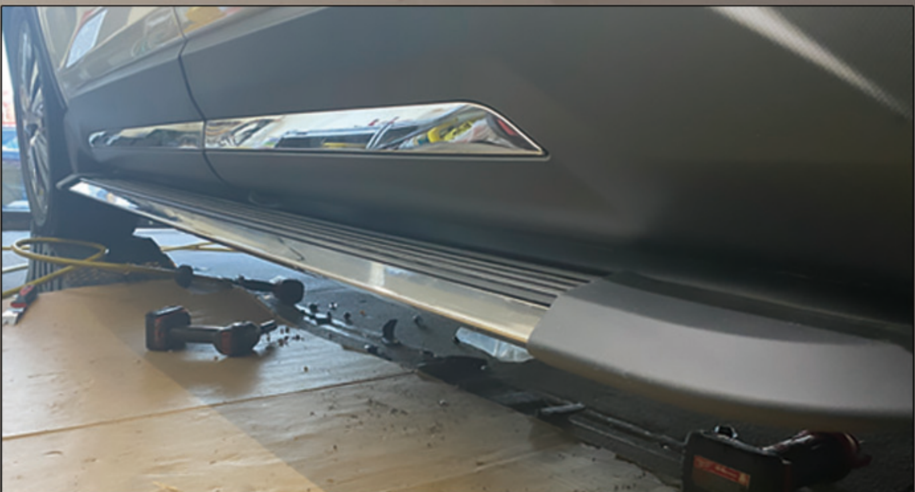
13. Complete the pedal installation.
