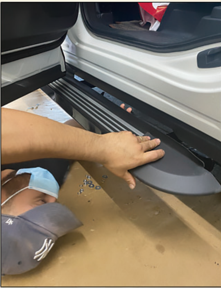
11. Reconfirm the installation height of the pedal.
