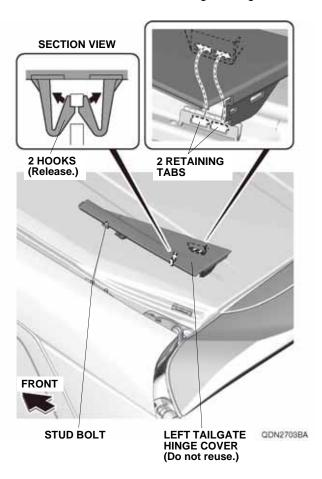
6. Remove the two clips from the two stud bolts on the roof.
