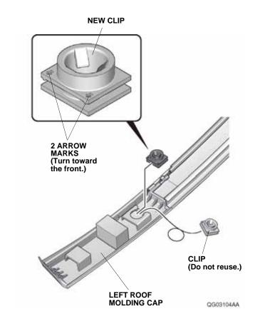
11. Install the left roof molding onto the stud bolt.
