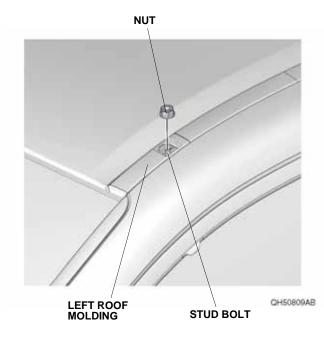
3. Remove the left roof molding as shown.
