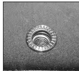
(Fig 6) Example of fully installed 6mm Insert
