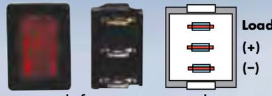
Mini switch for monitor panels, waterpumps, appliances. 16A @ 125V AC, 1/3 HP, UL, CSA, VDE. .82" x .60". Cut-out: .76" x .50".
