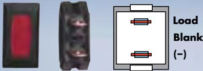
Standard indicator lamp, water heater, monitor panels illuminated in the "on" position. 10A @ 14VDC, UL, CSA, VDE. 1.23" x .68". Cut-out: 1.125" x .55".
