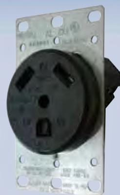
30 Amp, 125 Volt, NEMA TT-30R, 2 Pole, 3-Wire, Flush Mounting Receptacle, Straight Blade, Industrial Grade, Grounding, Side Wired, Steel Strap, Black.
