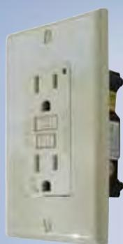
With reset button and LED light indication of no power, miswire or end of life indication when unit is not longer capable of providing GFCI protection. 15A or 20A, 120VAC with maximum interrupting Capacity of 2,000 Amps. UL Listed, CSA approved and complies to NEC, CEC and OSHA.
