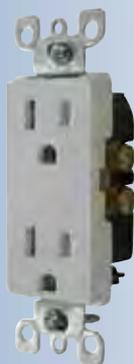
15 Amp, 125 Volt, NEMA 5-15R, 2 Pole, 3-Wire, Decora Duplex Receptacle, Straight Blade, Residential Grade, Grounding, Quickwire Push-In and Side Wired, Steel Strap. UL and CSA listed.
