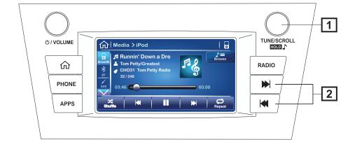
1 Tuning Knob - switch to next available channel, depending on direction of rotation. (Tuning knob may not be available while radio is loading channel list.)
