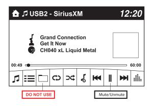
On the radio or steering wheel: Touch "Track Seek " " or "Track Seek " " to switch to next available channel. Long Touch on "Track Seek " " or "Track Seek " " to switch between Presets.
