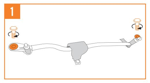
First please tighten the screw with a force of 10 Nm at the fixing points top left and right.
