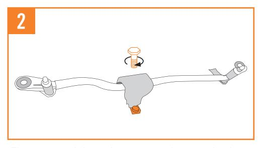
Then please tighten the screw at the lower holder with 10 Nm as well.
