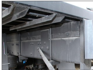
Structural C-channel Long Sills (ILO I-beam)
