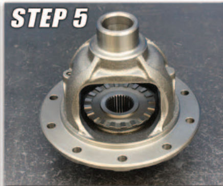
STEP 5 Install side couplers into carrier case
