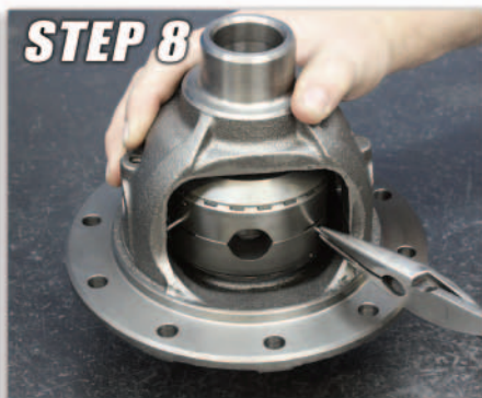
STEP 8 Align the center drivers to correct position & remove retainer wires
