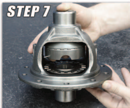
STEP 7 Install center driver & spacers
