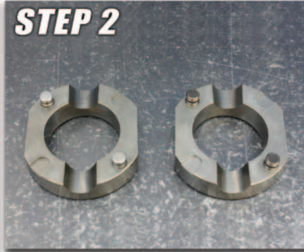
STEP 2 Install alignment pins/springs into driver holes
