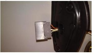
6. Re-plug wire harness and install back on door with three Phillip screws.
