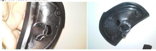
3. Insert wiring harness from the back side and pull through until the boot end engages the rubber plug attached to the wire harness.
