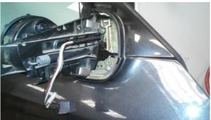
7. Reinstall mirror body covers as originally placed.
