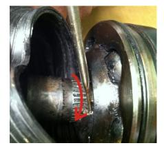
• Once a sufficient amount of the metal retainer key is exposed the remainder can be withdrawn with a pair of pliers.
