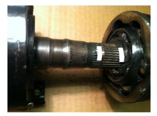
• Clean and lightly lubricate the splines and press together the shaft sections making sure to stop at the indexing paint mark.
