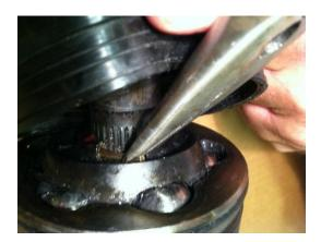
**Note:** Once the key if sufficiently located into the slot it may be possible to carefully tap the end of it with a suitable drift to push the remainder home.
