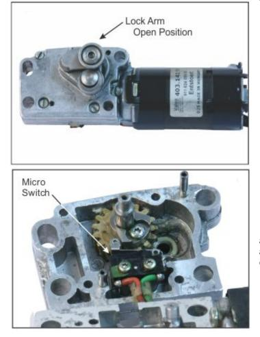
Carefully pry off upper cover exposing the gear set and miro-switch taking care not to change the lock arm position. <u>Note:</u> the locking arm will move freely once the gears disengage.
