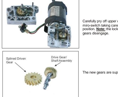
Carefully pry off upper cover exposing the gear set and miro-switch taking care not to change the lock arm position. Note: the locking arm will move freely once the
