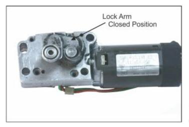
Starting with the top in the open position and remove damaged motor from car.
