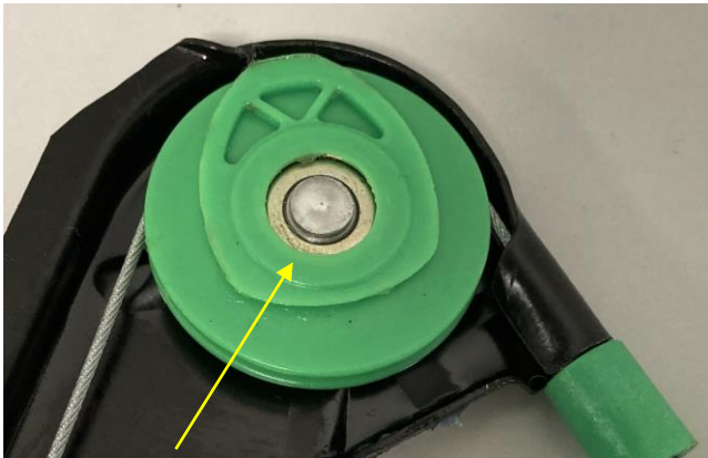
URO Pulley: Green plastic Pulley with integrated Ball-Bearing , which reduces friction and increases strength in rotational axis. Upgraded assembly compared to OE.
