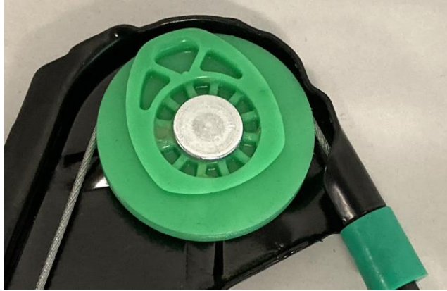
OEM Pulley: Green plastic Pulley pinned to steel frame, lubricated with grease.
