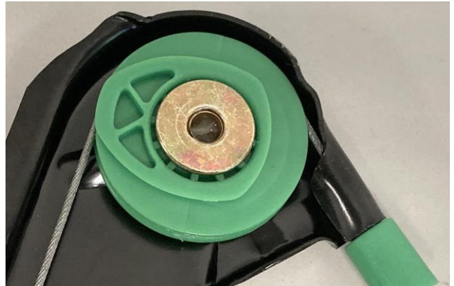
BRAND X Pulley: Standard offering green plastic Pulley, pinned to steel frame, lubricated with grease.
