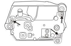
Step 3 – Remove upper shift cover (steel) attached by (2) T10 & T20 Torx screws.
