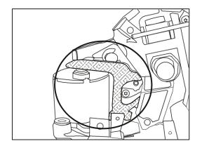
\*Note: there are 2 styles of shift park levers which are differentiated by the width of the hinge pivot base. Either a 5mm or an 11mm base may be fitted. This is a running change and not defined by a specific year or chassis. A quick inspection of the existing plastic lever in the shifter may be required before ordering the correct part.
