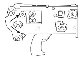
Step 6 – Using a suitable drift, remove fulcrum pin on remaining piece of broken plastic shift lever.
