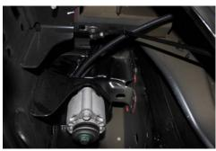
11. Once they reach the Passenger Fender well they will run up the back side of the fender to the engine compartment near the battery and ECU.
