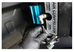
10. With the Compressor assembly and Lines bundled in the bed we can move on to routing the power cables. Feed them along the frame rail above the Body Mounts.
