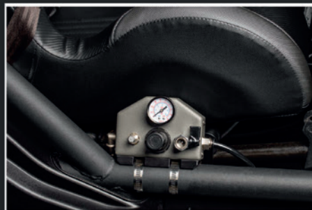
Tube Mounted ADS Controller
