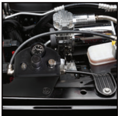
Part # 210-0717 GEN 2 Jeep Jk 4 Tire Inflation System On Board ADS Front Engine Controller Box
