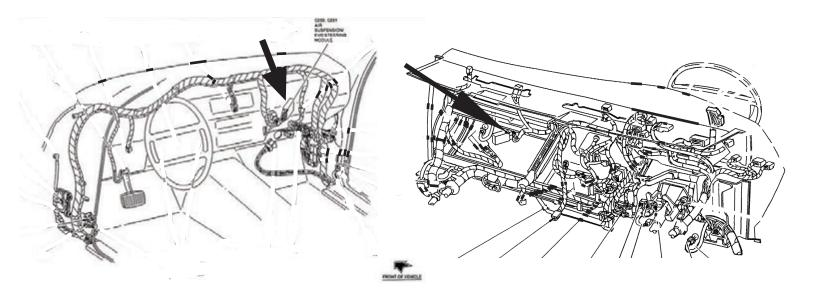
2. Behind the glove box, mounted to the heater plenum is a connection with two plugs, one GRAY, one BLACK, or both GRAY, each about 2". On the BLACK or TOP connector, midway, is a DARK GREEN/LIGHT GREEN wire (this is pin #11). Cut this wire to disable the "Check Air Suspension" light. Cut as far from the plug as you can should it ever need to be reconnected/spliced. Reattach the glove box.
