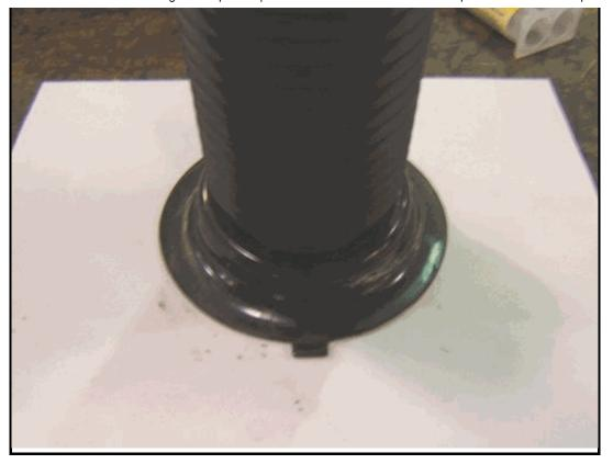
5. Glue the dust boot (shield) to the upper spring seat as shown using the above recommended adhesive. Allow to cure thoroughly.
