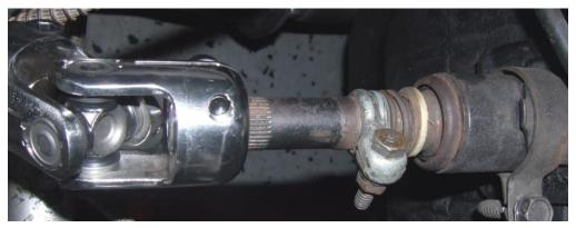
9. With upper u-joint on column with pinch bolt running across the flat on the shaft. Raise rack and pinion assembly up in between the frame rails. Line lower u-joint up with the splines on the pinion. Slide u-joint onto pinion.
