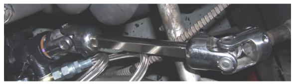
11. To finish your Corvette installation, please use the instructions that came with the Rack & Pinion. Do not tighten pinch bolts on u-joints at this time.
