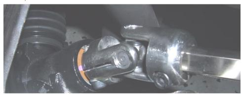
10. U-joint orientation is very important. When bolting intermediate shaft assembly into place. Install the joints 90 Degrees off of each other. This is important as it will reduce "BUMP", the hard points of rotation in the steering.
