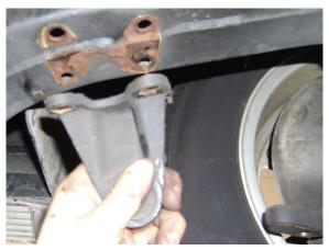
4. Remove stock steering linkage from vehicle.
