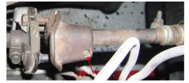
7. From above vehicle, measure 2 3/8" from the end of the steering column shaft and make a mark on shaft. Trim end of shaft off at 2 3/8" mark.
