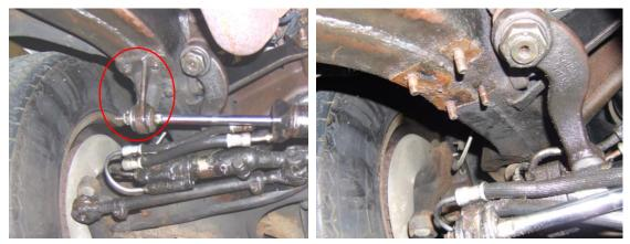
4. Remove stock steering linkage from vehicle.
