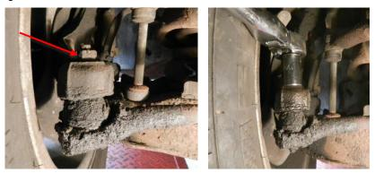
2. Remove the nut holding the pitman arm to the center link.
