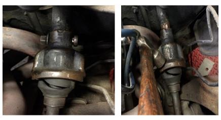
**9.** Remove the Hydraulic pump from the block. There are 2 bolts, one next to the header and one in the front of the block.
