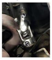
6. Install the longer steering shaft into the U-Joint.
