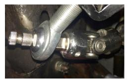
5. Install the U-Joint onto the steering column shaft. Tighten the set screw and nut flush with each other.
