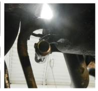
**6.** Remove the pinch bolt that connects the steering shaft to the gear box. Once loosened slide the steering shaft towards the steering wheel.
