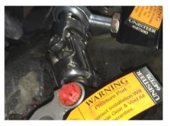
4. Install the shorter shaft into the U-Joint.
