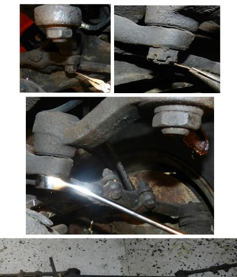
4. To remove the gearbox, the steering wheel shafts have to be disconnected. This is done on top of the car. There is a pinch bolt that connects the shaft to the steering gearbox. The bolt is a 12-point bolt head. Loosen the pinch bolt and proceed to the gearbox. To remove the gearbox there are four bolts. Remove three bolts and while removing the fourth one support the gearbox.
