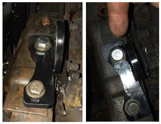
3. Now that the support is on apply the part 8050300 to the rack and pinion male shaft. Tighten the bottom allen head bolt. Next screw in the shaft support. This length may depend on angle. Screw it in and apply the angle to ensure it won't bind or hit anything. Once the desired thread length is found, apply the Jam nut and tighten. Measure the 10 5/8 long steering shaft and slide through the support into the swivel with rectangular end into the swivel.
