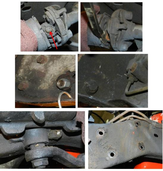
5. Once the gearbox is removed, the steering shaft can be removed. Remove the coupler at the top of the column. Loosen the nut then the stock shaft can be removed.
