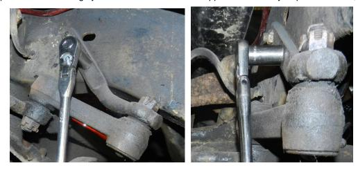
3. The next component to be removed is the center link connecting to the gearbox. This component has a cotter pin in it to be removed. Then the nut can be removed with a wrench or ratchet. This may have to be tapped out with a hammer. The linkage should then be removed from the vehicle.
