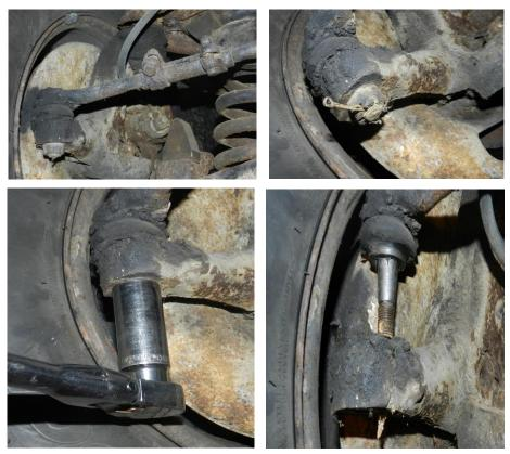
2. The next component to be removed is the idler arm. The idler arm is just a support bracket that supports the linkage and hold creates a swivel point on the steering system. 2 bolts and 2 nuts support it. This may require a wrench, ratchet and socket.
