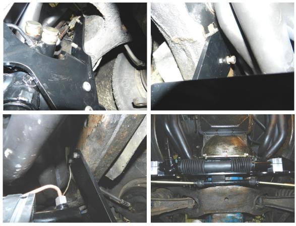
17. Once the rack is in place leave the bolts loose and install the shaft and u-joint from the rack and pinion to the steering column with the u-joint already on it. Slide the shaft onto the u-joint on the column and snug the pinch bolt. Run the shaft down to the rack, with the rack u-joint on the shaft, raise the rack into place to spline the lower joint to the pinion.
