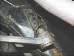
4. Remove tie rods from spindles.
