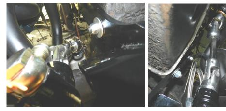
18. You can now torque the mounting bolts for your rack to 65 ft. lbs. Then torque the u-joint bolts to 40ft lbs
