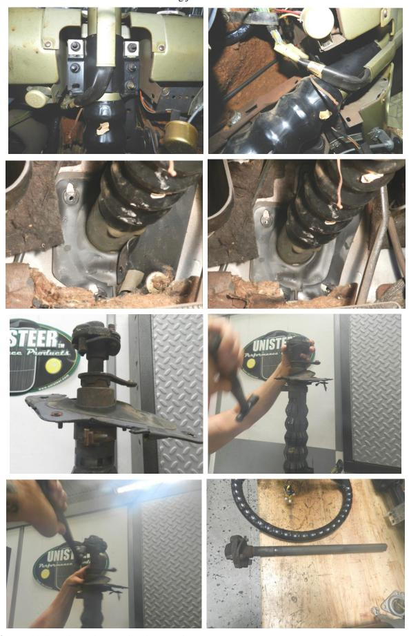
**NOTE:** This is a slip shaft, and will slide out of the column.
