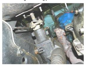
2. Remove the cotter pins and nuts from outer tie rod ends.
