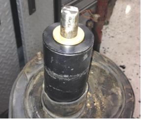
**NOTE:** You have to align the stock shaft and make sure the bearing slides easily over the shaft. Damage to the needle bearings and bindings of the shaft will occur if note done properly.
