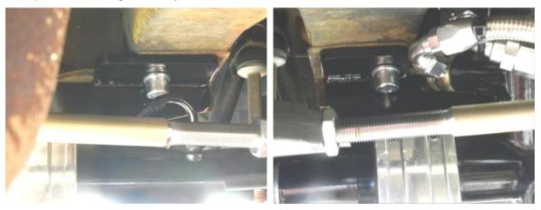
15. Install the outer tie rod ends and tighten to 45 ft. lbs. Adjust the toe by eye so you can drive to an alignment shop. Tighten down the jam nut. Toe is adjusted with everything together by leaving the jam nut loose and turning the rack inner end. Outer ends are installed with the curve pointing towards the rear of the car.
