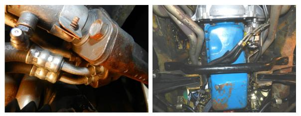
3. While you are under the car pull the cross-bar off by taking off the one bolt on each side. This is where the rack mounting bracket will be mounted later.
