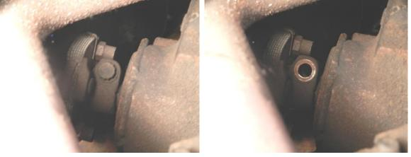
2. Remove the cotter pins and nuts from outer tie rod ends and remove tie rods from spindles. Unbolt the Idler Arm from the frame. Unbolt the power assist assembly from the frame and unbolt the four bolts on the gear box. Last remove the hoses and then remove the entire steering linkage.
