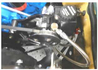
11. Route the lines together down to the rack and pinion where they will connect. Make sure they have a safe distance away from anything hot, sharp, or moving.
