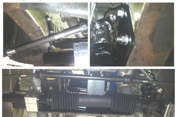
9. You can now eye up your tires toward the straight position and connect your outer tie rod ends and install supplied cotter pins. Install grease fittings.
