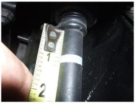
2. Cut steering shaft on 1" mark and remove the lower part of the stock steering shaft.
