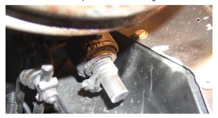
3. Install new intermediate shaft kit on the rack using the lower u-joint. Slide the upper u-joint onto the exposed remaining column shaft. Slide the intermediate shaft into the upper u-joint. Note: make sure end of existing steering shaft is flush with inside of u-joint. Tighten set screw on u-joint against the shaft with the u-joints phased 90 Degrees off one another.
