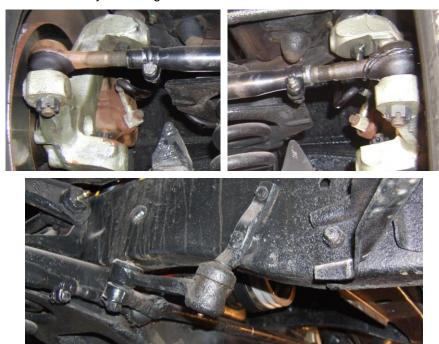
2. Remove the pinch bolt from the input shaft on the steering box. This will allow for the gearbox to be completely removed after removing the three bolts holding it to the frame.
