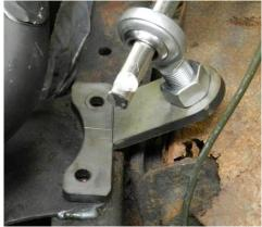
6. Insert middle joint with lower shaft so that the yokes on the joint are facing the same direction as the lower and upper (marked in red in the picture). You will have to trim the lower shaft to fit. Make sure all joints are lined up correctly and the support bearing is adjusted out where it needs to be before making your cut. Then grind a notch for the pinch bolt. Re-assemble the shaft kit, check for binds, and then tighten everything down.
