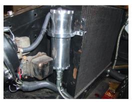
4. Hook power steering lines up, Pressure line goes to top port (blue fitting) on rack housing. Return line is the lower port on the rack (silver fitting) which goes to lower #6 fitting on the remote reservoir. Large #10 line goes from large port on the reservoir to nipple on pump and secured with supplied hose clamp.
