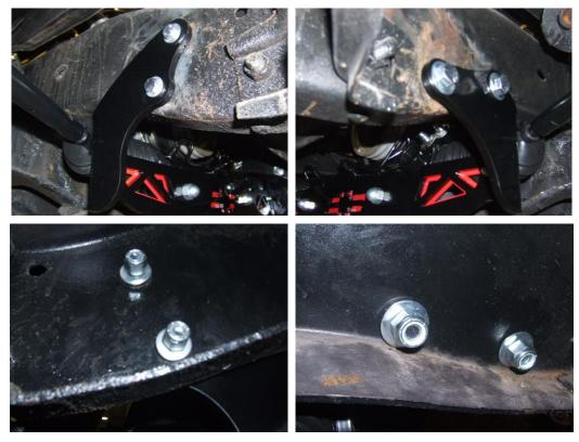
6. With new R&P system bolted into truck, its time to hook up the steering. Bolt tie rod ends into spindles.
