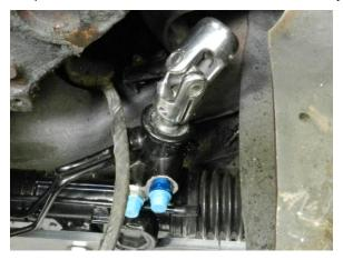
3. Slide upper u-joint on column so that the yokes are lined up in the same way and insert pinch bolt.
