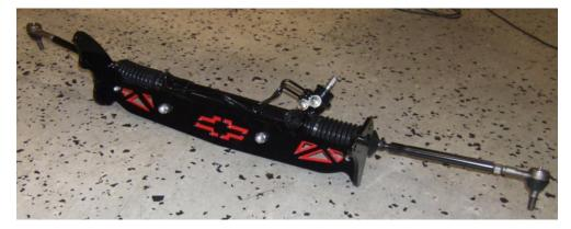
5. Now to install your new kit. With supplied hardware (2: ½-13 bolts and 2: 3/8-16 bolts). Bolt new R&P kit up into frame. Note: ½" bolts are used in drivers side and 3/8" bolts are for passenger side.
