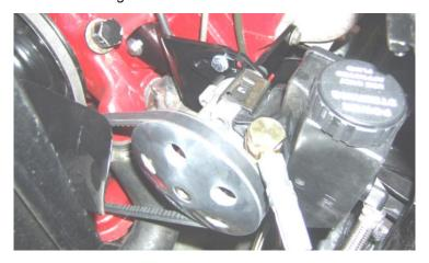
11. When that is complete you are now ready to take a measurement on your belt. We usually take a tape measure and go around the pulleys to get a rough idea and then get a couple of belts that are around that measurement.
