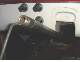
3. Next remove the steering box bolts on the driver side of the frame and remove the gearbox entirely with the shaft. Next you will need to modify your column tube. First measure up from the bottom of the column tube that was connected to the gearbox 3" and cut off that portion using a tube cutter or band saw. Make sure to do this accurately and squarely.
