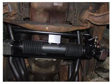
9. Then install the 2 bolts on the passenger side from the outside of the frame in and install the flat washers and lock nuts but do not tighten.
