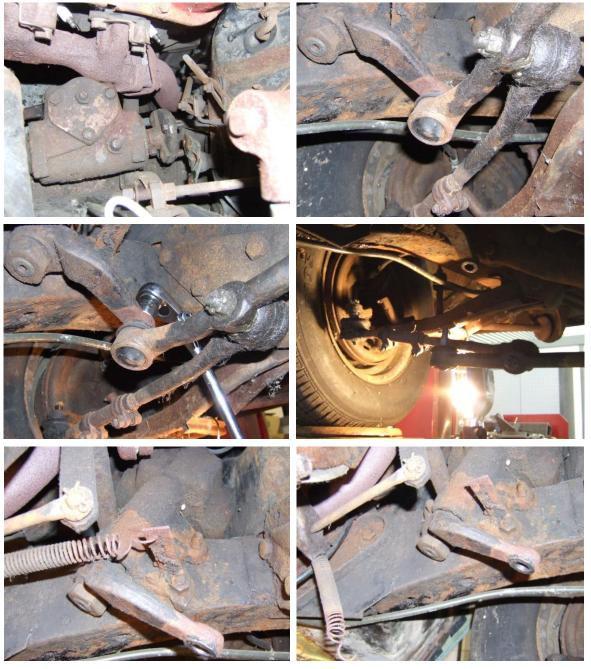
4. Remove the 2 retaining bolts on the idler arm assembly. Remove the idler arm and the rest of the steering linkage.
