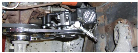
17. Next install the pressure and return line. Note the pressure line has the 1 female end on each end. That line runs to the lower port on the rack and the top port of the power steering pump. The return hose goes to the upper port of the rack and the slip on end goes over the reservoir plastic nipple with a hose clamp. Tighten all lines to 15 ft lbs. Make sure your line routing is good. Do not route lines so they kink or come in contact with hot or sharp surfaces.
