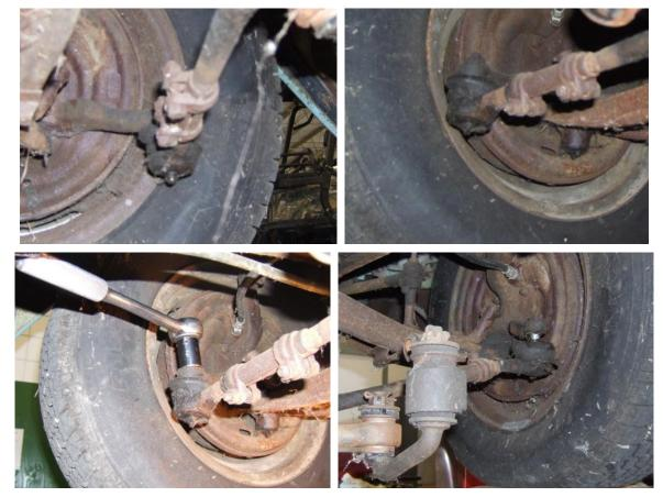
3. Remove the steering column pinch bolt at the rag joint. Remove the center link point at the pitman arm. Remove the three retaining bolts that hold the gearbox to the frame. Remove the gearbox.
