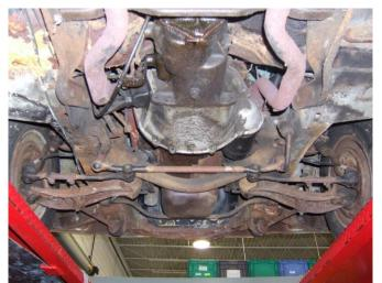
2. Remove front tires. Remove outer tie rod ends, cotter pins, and retaining nuts. Remove outer ends from spindle.
