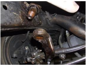
3. Remove the steering linkage from the car. If the car has power steering remove the lines from the assist unit and remove it with the linkage.
