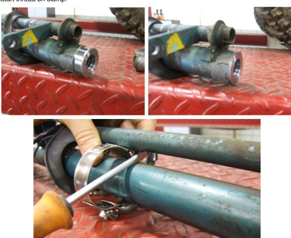
9. Once that is done you can reinstall the column tube in place. Using the new floor plate align your column using the stock u clamp at the top under dash to hold it in place while you assemble the floor plate. Before installing the floor plate you will need to take a pair of pliers and bend the 3 tabs on the plate toward the inside of the car. These tabs will now support the column at the firewall and allow the clamp on the column to squeeze the tabs on the plate.
