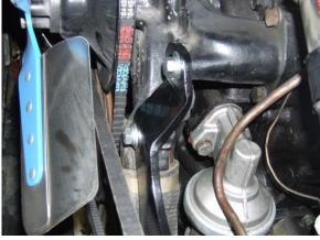
14. Once you have your belt installed and tightened you will need to connect your lines. The return line goes to the plastic nipple on the side of the reservoir. The pressure line goes to the fitting on the top of the pump. Once the lines are on and tight you can top off the reservoir with power steering fluid.
