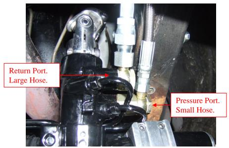
13. Your kit comes with a new pump and bracket. If your car had power assist you can remove the stock pump and bracket from the engine. Your new bracket goes in the same place and uses the hardware provided in the kit to install it. You will need to take a belt measurement around the pulleys and purchase a new v-belt. If your car did not come with power assist you will need to purchase a crank pulley from a Ford shop or an aftermarket company.
