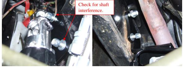
9. Now install your upper and lower u-joint and assemble the intermediate shaft assembly. Slide the provided plastic washer over the column shaft and install the column joint. Next install the lower pinion joint on the rack. Lower the driver side of the rack to install the intermediate shaft. Note when doing this step make sure you orient the u-joints **out of phase** 90 degrees opposite of each other. Once connected tighten the main mount bolts to 50 ft lbs.
