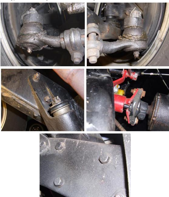
3. Remove the steering linkage from the car. If the car has power steering remove the lines from the assist unit and remove it with the linkage.
