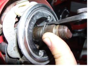
5. From under the hood slide the steering shaft out of the column tube as far as you can get it and cut it off with a reciprocating saw or similar saw. Once removed slide more of the stock shaft out of the column and cut off another piece. Repeat this
