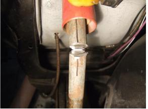
Once the complete shaft is out you can now install the supplied bearing into the bottom of the column. Do this by centering the bearing inside the tube and tapping it in with a hammer evenly around until it seats against the tube.
