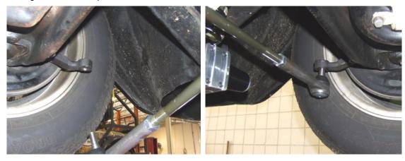
12. From under the car you can install the pressure and return line in place. The larger hose is the return line and goes on the top port closest to the pinion. The smaller line is the pressure line and goes to the lowest port on the rack. Route the lines up the frame in the shortest route to get to the new pump.
