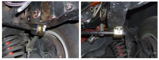
8. You are now ready to install the rack and pinion. Your rack has come assembled to the mounting bracket. Put the rack and bracket up in place and using the new supplied hardware, install the bolts on the driver side and passenger side where the steering box and the idler arm used to be and let the bracket hang. Install the washers and nuts and torque to 45 ft. lbs.
