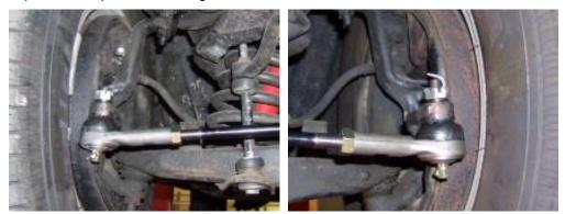
Alignment Specs: Toe: 1/16" for radial tires & 1/8" for bias ply Camber: 0-1/4" positive (1/2" max) Caster: +2° on both sides
