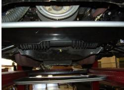
9. Install the heim joint by threading it into the hole and start with the joint about ½ way through the threads for adjustment. Slide the support bracket over the driver side mounting bolts and leave loose.
