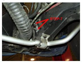
8. The driver side uses the supplied 7/16 hardware and uses 2 of the 3 mounting holes where the gearbox used to be. Once the rack is hanging in the car leave the hardware loose. Making sure the rack is in the center of the car and the pinion is also centered you can now install your steering shaft support bracket.
