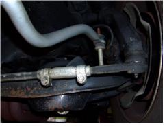
4. Remove stock steering linkage from the vehicle. Remove the 3 bolts on the outside of the driver side frame that hold the gearbox to the vehicle, then remove the entire gearbox. Note: this may require wiggling the box off of the steering shaft.
