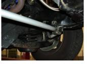
5. From under the hood, remove the pinch bolt at the top of the steering column. Slide the stock shaft off of the column.
