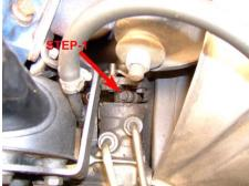
2. Remove power steering pump and brackets from engine. Disconnect pressure and return line from pump.
