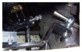
10. Install the upper u-joint onto the column shaft and paying attention to the flat surface of the shaft, place u-joint set screw over flat. Locktite the set screw and tighten to 25 ft lbs. Then tighten jamb nut.
