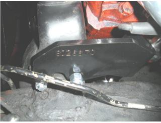
8. Place supplied (Ididit) column in place with inboard firewall plate over steering column tube (it wont fit after the column is thru the firewall). Begin by installing the column clamp under the dash, directly behind the where the steering wheel will be.
