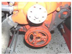
4. Remove the lower fan shroud.
