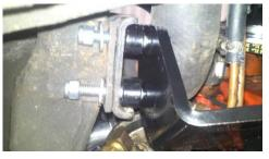
5. With kit bolted up in chassis. Notice that on the mounting bracket, there are two round holes and two slots. Rack slots allow adjustment of the column shaft bracket. Fasten the rack bracket in a position that allows a straight shot from the pinion up thru the steering shaft support bracket.
