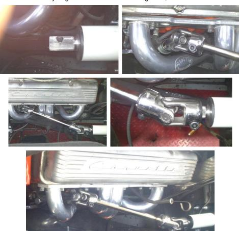
13. Make sure entire shaft assembly is routed without interference. Tighten u-joints and the shaft support bracket. Make sure the jam nut on the hiem joint is tight as well. Tighten rack bracket bolts down to the suggested: 36 ft lbs.
