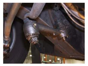
7. Remove the bolts that retain the gearbox to the frame and remove the gearbox. Once the box is out, you can set it aside you will not need this again.
