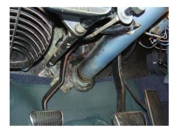
4. Remove the column tube assembly from the vehicle. You will need to reuse the column plate or screws. Be sure to save the pinch bushing at the top of the steering shaft and column tube, you will need to reuse this piece.
