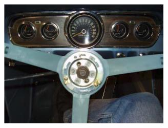
2. Remove steering wheel center nut and remove steering wheel assembly. **Note:** A puller may be required to remove wheel.
