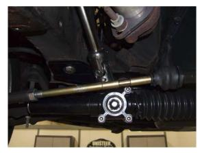
11. Next, you need to modify the column and tube assembly. Using a band saw or a sawsall, cut off the rag joint as close to the weld as possible. Once that is done, clean the steering shaft of rust and scale. Install supplied bearing over shaft and into column tube. Tap the bearing in with a small hammer until seated in the column. Measure down 1 ¾ inch from the flat surface of the bearing. Mark the shaft and cut on the line.
