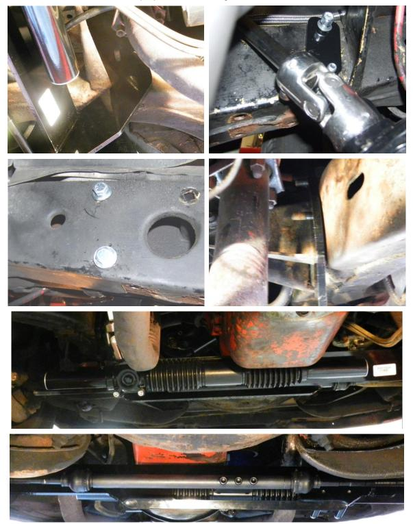
3. Thread lock nuts and tie rod ends onto the inner tie rods.
